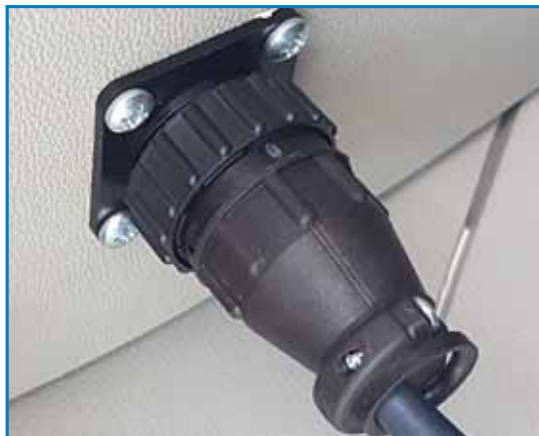
Quick exchange connector to change easily between different gas/brake controls
