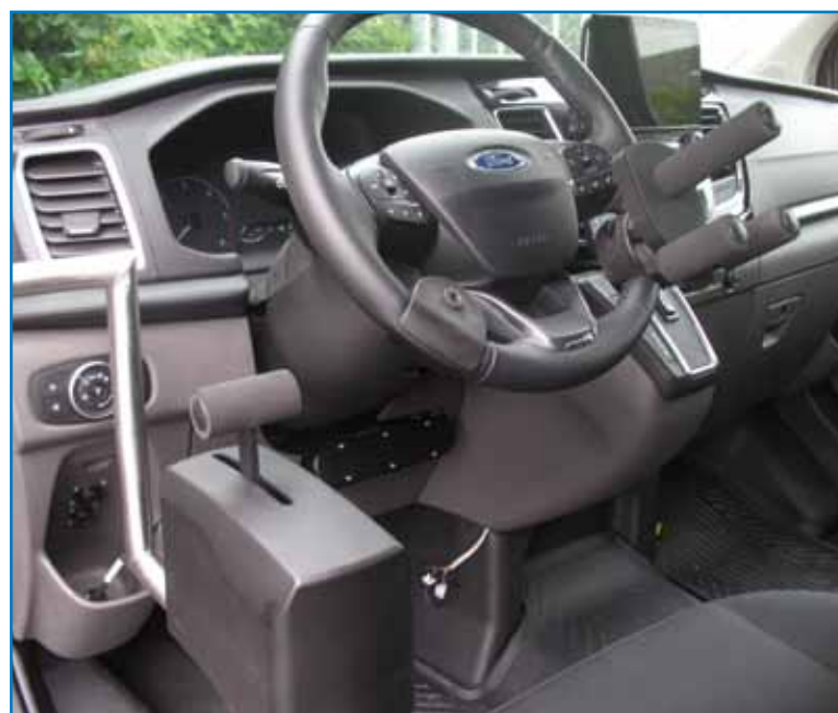
Gas/brake lever with T-grip combined with Bever 3-pin device
