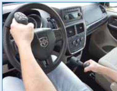
Right-side hand control mounted on SmartBrake floor bracket
