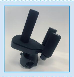
The 3-pin device is for the driver with adequate arm strength, but minimal grip strength and / or reduced wrist stability. It supports the hand and wrist and keeps them comfortably in position. The tri-pin device consists of 3 legs. The front leg has a fixed position, the rear legs can be adjusted inward, outward, forward and backward. This allows the tri-pin steering grip to be perfectly adjustable to fit the shape of the hand.
